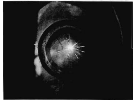
Fig. 3 Cathode spot of graphite and droplet emission.
