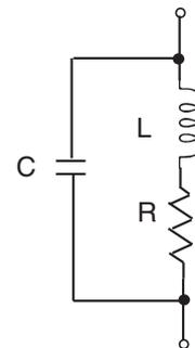
Fig. 2. Schematic of the equivalent circuit of MWCNC.
